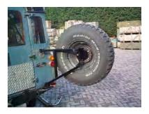
Place the carrier in position with the bottom bracket straddling the rear cross member to body lug. Ensure that the top hinge bracket is level with the top of the body capping on the rear tub. (N.B If the wheel carrier is being fitted to a vehicle with a rectangular rear fog lamp, this may require rising slightly in order to provide clearance for the diagonal tube).
