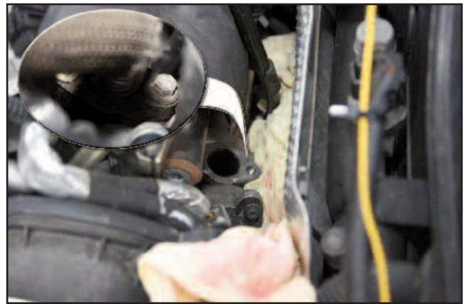
EGR pipe flange bolts
