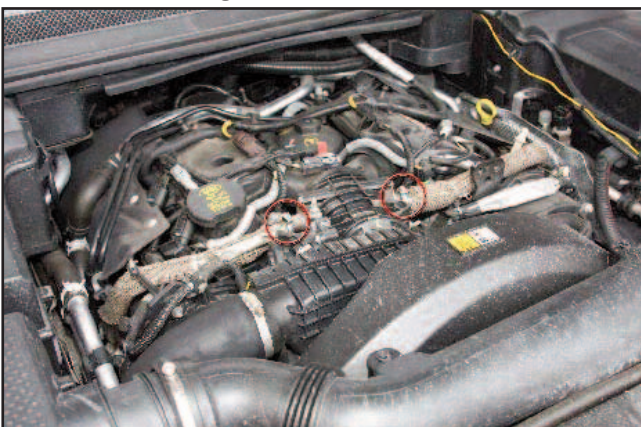
EGR pipe clamps
