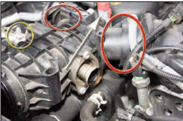
Raising the butterfly housing. It will swivel where circled but don't go much or you'll break the plastic that is holding the connector (arrowed) to the back of the 'Y' shaped duct.
