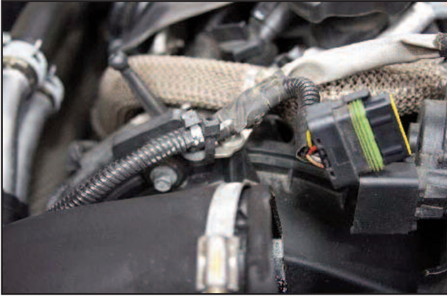
Tie-wraps – right hand EGR pipe bracket
