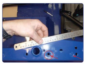
Using a straight edge draw a line across the remainder of the bulkhead capping and cut off using a grinder. Remove any burs and sharp edges using a file. Drill out the 2 pop rivets shown then drill out the hole circled to 10.5mm.
