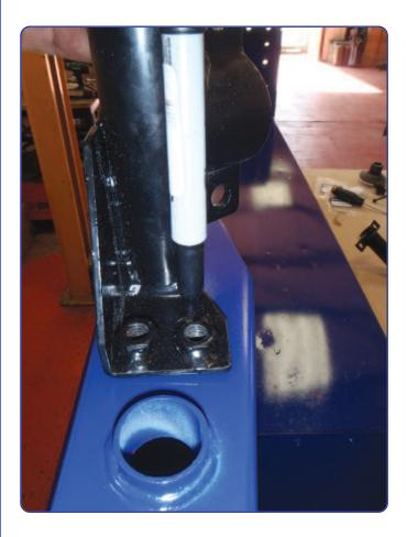
Once you have worked out which side bar is which, take the side bar from the opposite side and place it upside down on top of the side you are working on and align with the 10.5 mm hole you have already drilled and align the outside of the capping on the rear tub with the bracket.
