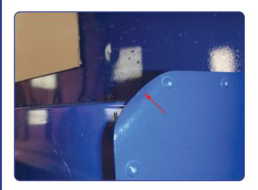
Using a circular object draw a radius of approx 50mm on the top corner of the wheel arch and cut this out.
