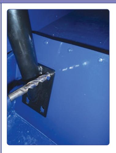
Fit the tube side brackets into position and secure at the top using the pan head bolts provided.
