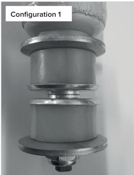
Pictures show the correct bush and washer configuration to the type of axle the shock absorber is being fitted to.
